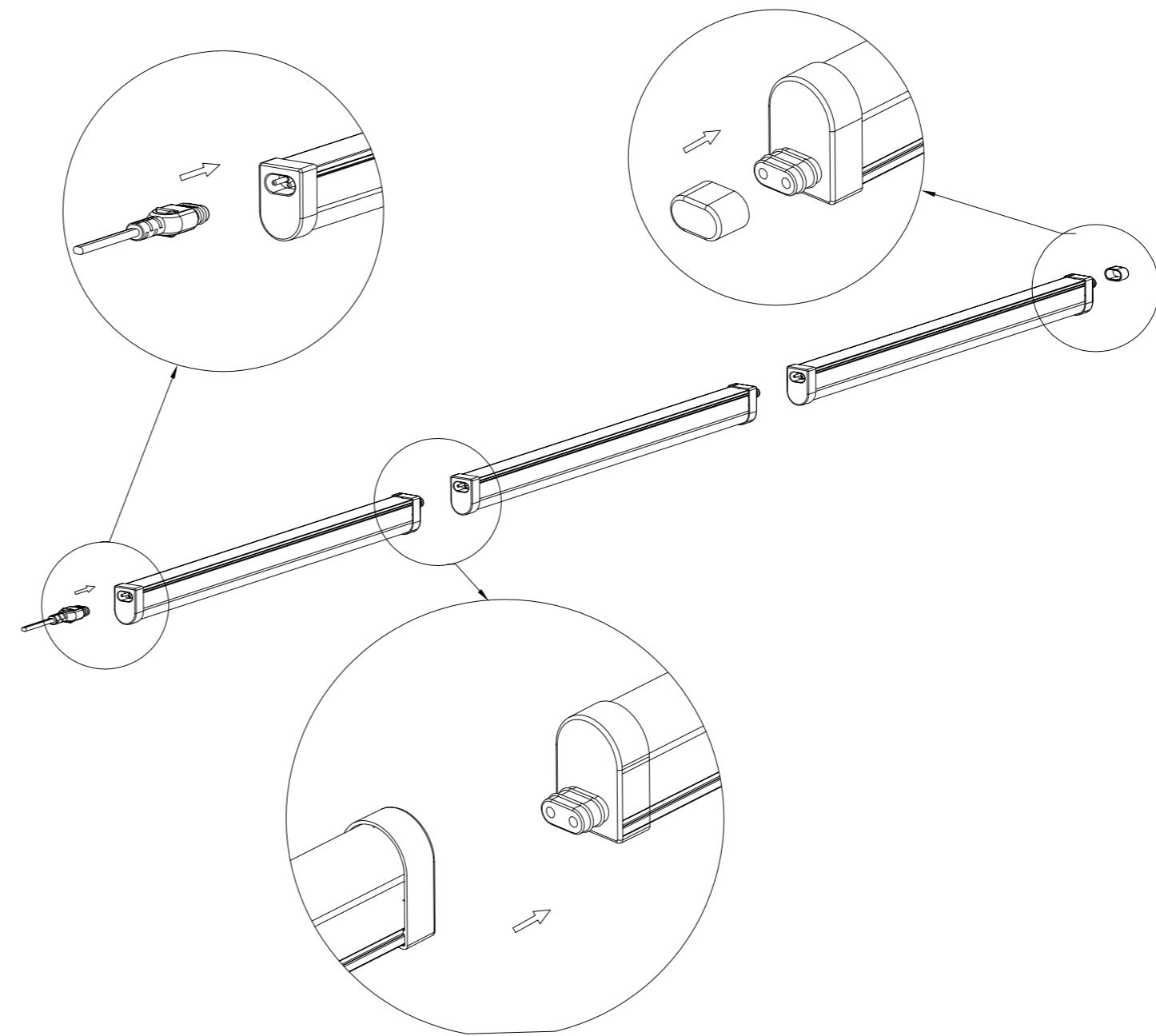
Step 2. Snap the lamp into clips.
