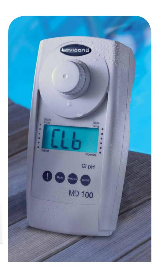
The MD 100 uses high quality interference filters with long-life LEDs as a light source in a transparency sample chamber.
