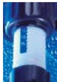
The injection rate is set by lining down the top of the adjusting sleeve with the desired ratio on the scale. The amount of injected concentrate is proportional to the amount of water coming into the Dosatron : i.e. Adjustment at 1% = 1 : 100 = 1 Volume of concentrate into 100 Volumes of water.
